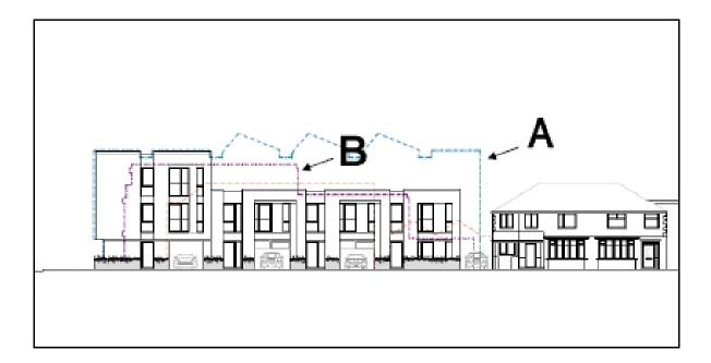
In terms of the massing, this has been broken up by using contrasting and recessed panels of cladding and brick and vertical glazing. This can be seen in the elevational drawings located earlier in this report.
